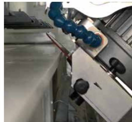
45 degree cutting Taglio a 45°
